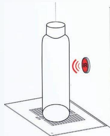
Infrared sensors are placed at the center of the console. Simply place a container (cup, bottle) on the support grid and let the sensors do the work. As soon as the container is detected, the water supply is triggered. To stop the distribution, just take back the container.
